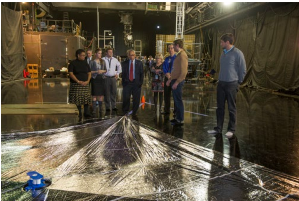
NASA Administrator Charles Bolden visited the Near-Earth Asteroid (NEA) Scout project at Marshall Space Flight Center on Dec. 14, 2015, in Huntsville, Alabama, where a team completed a half scale-solar sail deployment test. The test confirmed the folding technique, package efficiency, and the deployment mechanism for the solar sail.
